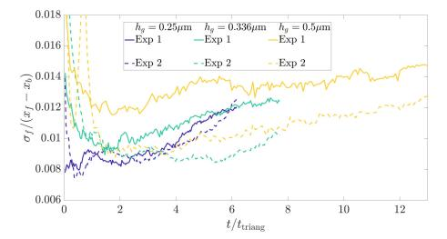
FIG. 5. The scale of the roughness of the density front  $\sigma_f(t) = \text{std}[x_f(y;t)]$ , normalized by the length of the density profile  $x_f(t) - x_b(t)$ , for two experiments at each of the three gravitational heights. Time is scaled by a rough estimate of the time it takes for the density profile to become (approximately) triangular,  $t_{\text{triang}} = 20$  min [see also (4)]. In the SM [15] we show the temporal evolution of the characteristic wavelength of the fronts.
